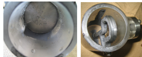
Fig.3: Remained contamination in the input coupler port (left) and HOM coupler (right) after a regular HPR (6MPa, 15min) with SRF single cell cavity at WG5-KEK.
