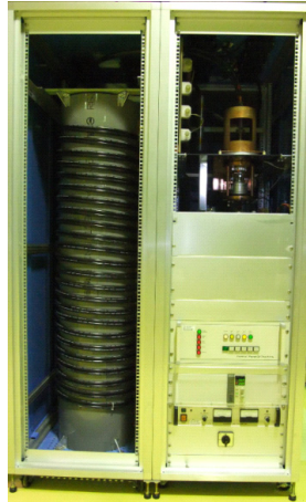
Figure 2: Photo of the PFN pulser test unit.
