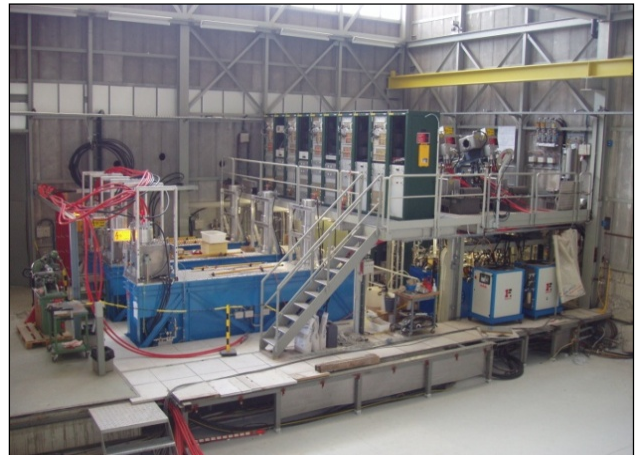
Figure 2: Kicker generators for KFA4 (right), 13 and 21.
