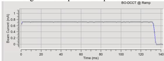
Figure 5: Current measured in the DCCT along the ramp showing no losses during ramping
