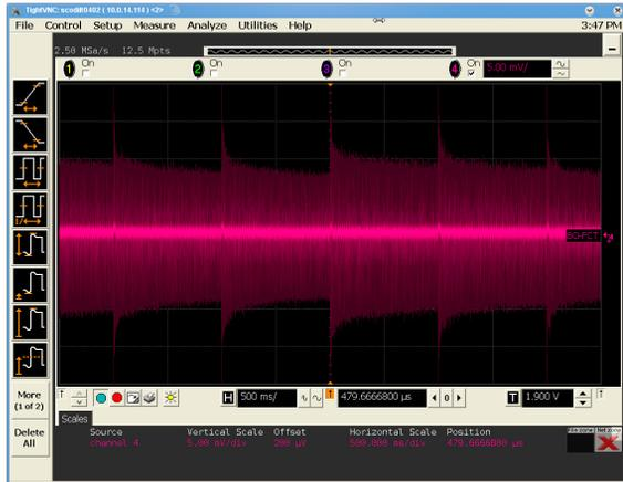
Figure 3: first stored beam in the booster. Several injections at 1 Hz are shown
