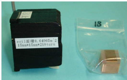
Figure 1: Pick up coils for the quadrupole magnet field ripple measurement.
