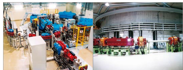
Figure 4: Proton (left) and proton/carbon (right) therapy system by Mitsubishi.
