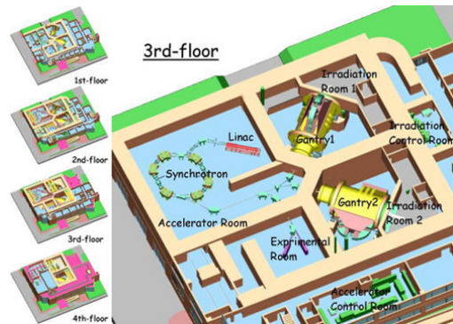
Figure 2: Layout of the proton therapy synchrotron by Hitachi for PMRC.
