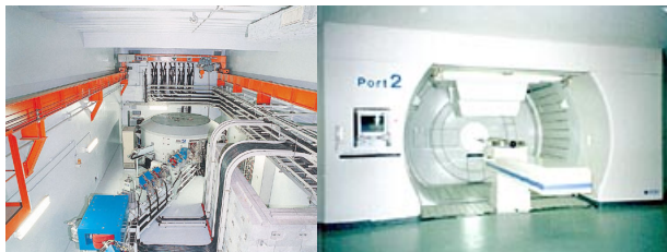
Figure 3: The cyclotron proton therapy system manufactured by Sumitomo, 230MeV cyclotron (left) and gantry (right).
