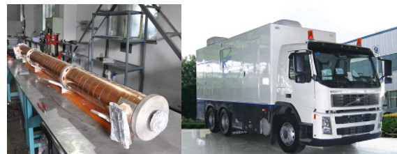
Figure 7: New electron radiation processing technology developed in China. The L-band 10MeV/40kW TW linac waveguide by IHEP (left), the mobile sterilization system with 2.5MeV/1kW SW linac by THU (right)
