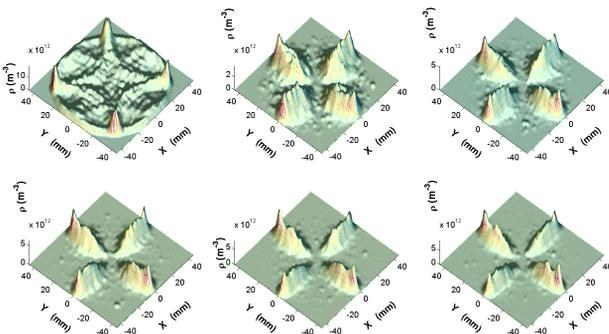
Figure 6: Evolution of electron cloud during the train gap; subsequent frames are separated by  $\Delta t=70 ns$ . Parameters used for simulation: bunch length  $15mm$ , bunch current  $1.3 mA$ , bunch spacing  $14 ns$ , field gradient  $0.517 T/m$ , peak SEY 2.0, energy at peak SEY  $276 eV$ .
