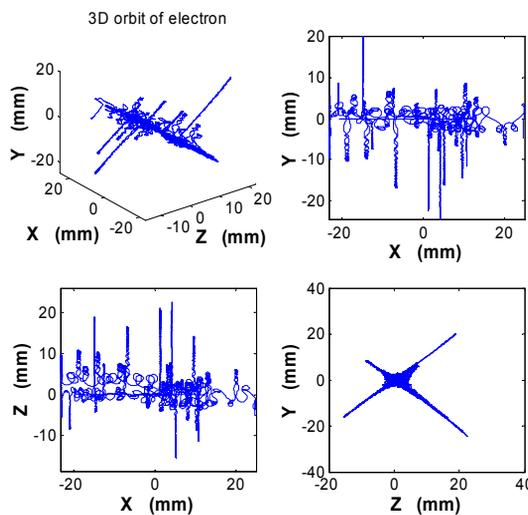
Figure 4: Example of an electron trajectory, which shows how the electron passes through the beam chamber horizontally.
