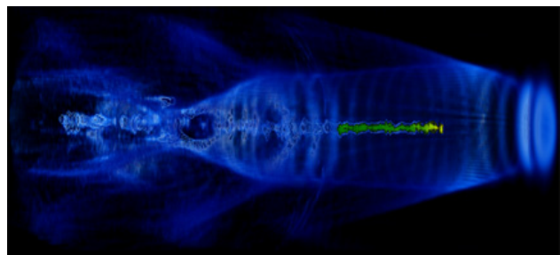
Figure 2: A three-dimensional VORPAL simulation models the self-consistent evolution of the wake resulting from a laser pulse and the acceleration of particles in a laser-plasma particle accelerator. Courtesy of G.H. Weber and C. Geddes.
