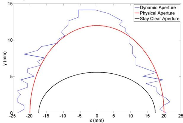
Figure 3: Booster dynamic aperture shown with physical aperture and stay clear aperture.
