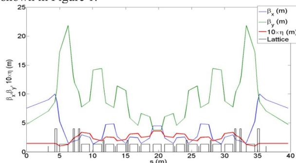
Figure 1:  $\beta$  and dispersion functions through one quadrant of the NSLS-II Booster Reference design.
