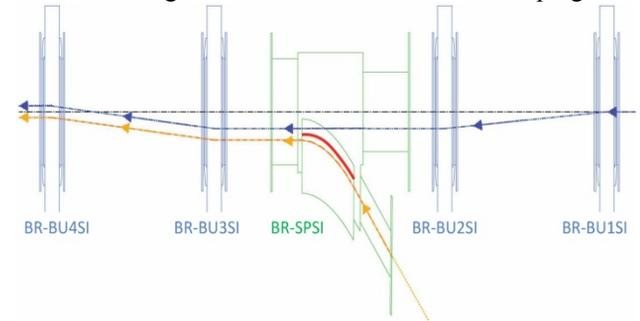
Figure 5: Injection of the second bunch train into the NSLS-II Booster.
