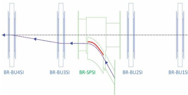
Figure 4: Injection of one bunch train into the NSLS-II Booster.
