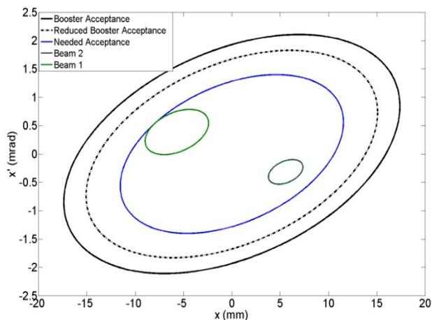
Figure 6: The booster horizontal phase space at the end of the injection straight after the injection of the second bunch train. Sufficient phase space exists for two beams to circulate.
