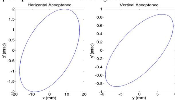
Figure 2: Horizontal and vertical stay clear aperture of the booster reference design.
