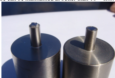
Figure 1: The cathode plug with original and recessed GaAs crystal. The left plug is the original, the right is the new recessed plug.
