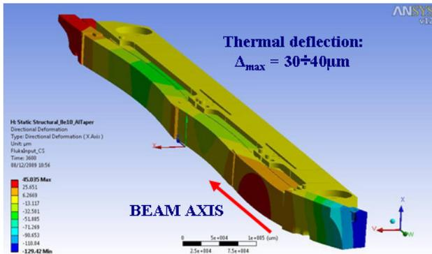
Figure 5: Thermo-mechanical analysis performed via FEM method. Jaw thermal deflection is about 30±40µm.
