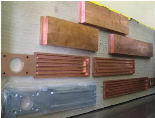
Figure 6: Main components of equipped jaw sectors. First Phase II prototype with GliCop Jaws.
