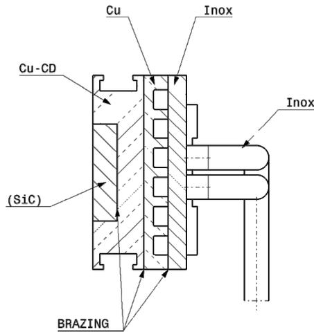
Figure 2: Phase II equipped jaw. The cooling system is brazed to the jaw. Two possible solutions: Cu-CD jaw and Cu-CD jaw with SiC inserts (both conductive and non-conductive options can be implemented).
