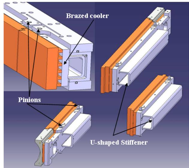
Figure 4: Equipped jaw sectors made up of jaw sector, cooling circuit with brazed cover and U-shaped stiffener..
