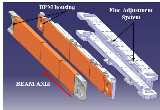
Figure 1: Phase II jaw assembly. Modular design including (from left to right) three-sector jaw, three-sector cooling circuit and back-stiffener with fine adjustment system.
