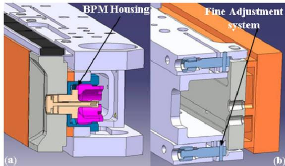
Figure 3: Cross-section of jaw tapering with housing and fine positioning system for BPM.
