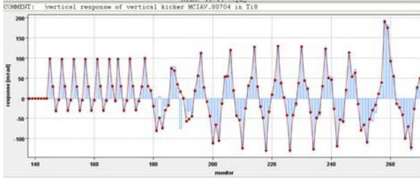
Figure 6: Vertical response from vertical kick at the TI 8 start. Beam from the left.
