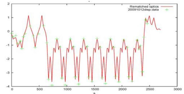
Figure 3: First order dispersion measurements (+) vs. model (continuous line), after the optics rematching.
