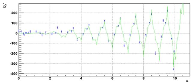
Figure 4: Second order dispersion measurements (+) vs. model (continuous line), after the optics rematching.
