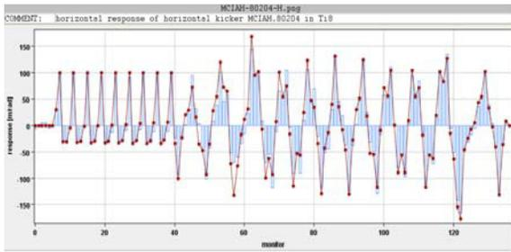
Figure 5: Horizontal response from horizontal kick at the TI 8 start. Beam from the left.
