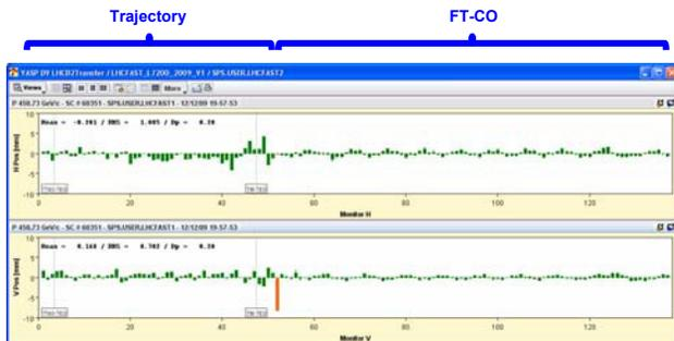
Figure 7: Steering application display showing the trajectory in the transfer line and the “first turn-closed orbit” in the LHC adjacent sector.
