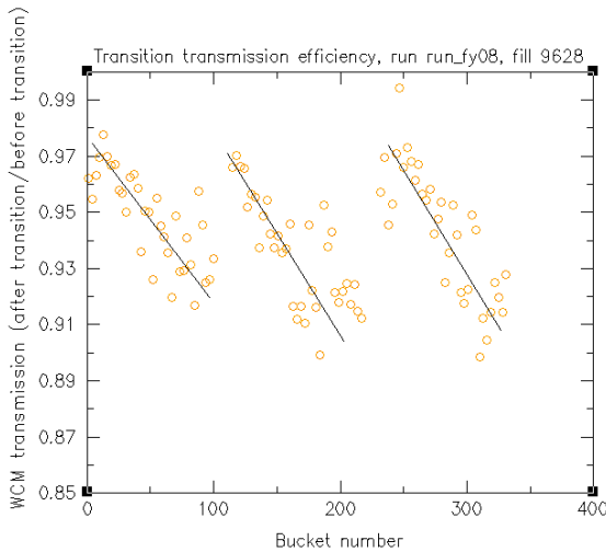
Figure 2: Bunch intensity transmission through the transition in dependence on bunch position in the train.
