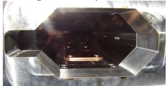
Figure 5: Installed electrode in the dipole vacuum chamber.
