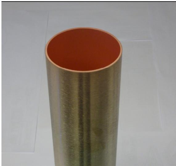
Figure 5 copper coated RHIC tube sample
