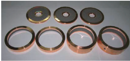
Figure 6: Cavities and disks with Kanthal coatings.
