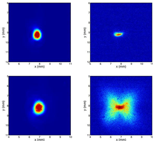
Figure 3: 795 nm laser image before (top-left) and after (bottom-left) U1; Electron beam image before (top-right) and after (bottom-right) U1.
