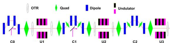
Figure 1: Schematic of the echo-seeding experiment
