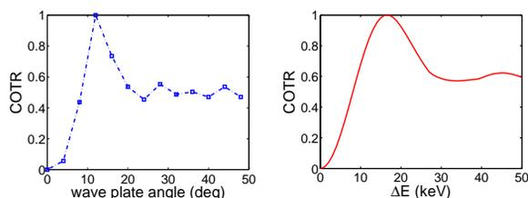
Figure 5: (a) Measured COTR peak intensity vs wave plate angle; (b) Simulated COTR peak intensity vs peak energy modulation amplitude.
