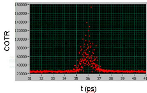
Figure 4: COTR intensity vs laser timing
