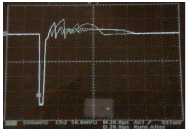
Figure 5: High voltage pulses as scope traces. After the main pulse of 5 us the thyatron can switch off in many different ways in the following 100 μs.
