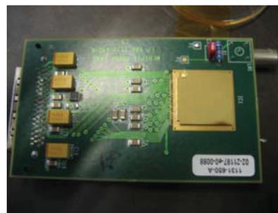
Figure 6: Spectrometric detector on basis of GaAs (Cr) pixel sensor with 256×256 channels of 50 μm resolution and Medipix chip.
