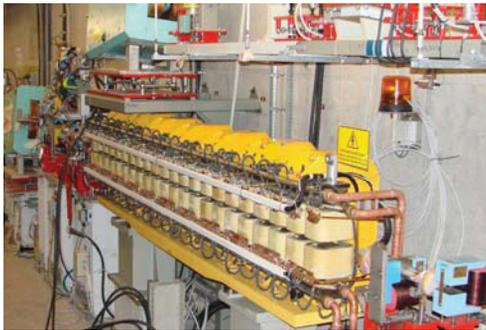
Figure 3: FLASH far infrared undulator constructed by JINR.
