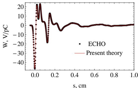
Figure 3: Wakepotential of a  $\sigma_z = 100 \mu\text{m}$  bunch.
