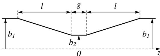
Figure 1: Geometry of an axisymmetric collimator.
