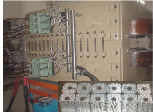
Figure 14: CSNS RCS dipole magnet and the stranded aluminium conductor (insert) fabricated in China (photo courtesy of Institute of High Energy Physics, CAS).
