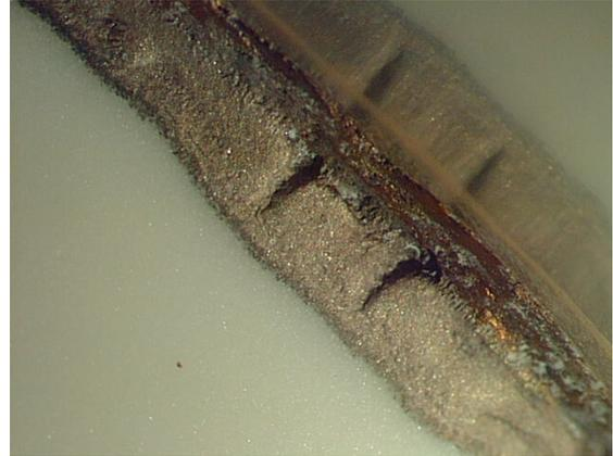
Figure 3: Active braze joint between the ceramic tube and kovar flange which has cracked.
