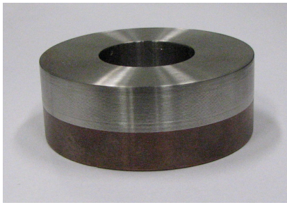
Figure 6: SS/Cu flange fabricated using diffusion bonding weld.
