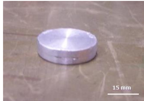
Figure 3: Al/Al diffusion bonding welded sample.
