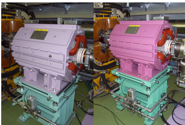
Figure 2: EQ and RQ magnets. (left: EQ1, right: RQ)
