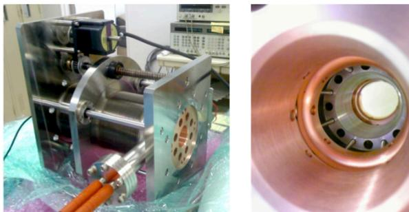
Figure 3: Pre-buncher chamber and its drift tubes.
