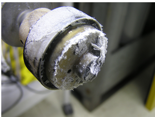
Figure 2: Paraformaldehyde generation in the coldbox. Here a picture from the cone of a hand valve of the internal N 2 -adsorber is shown.
