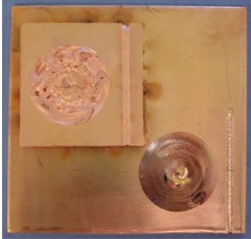
Figure 3: EB surface melting (overlapping spirals) and weld test (vertical lines) conducted on an OFE copper plate (lower right) and EBMed copper plate (upper left).
