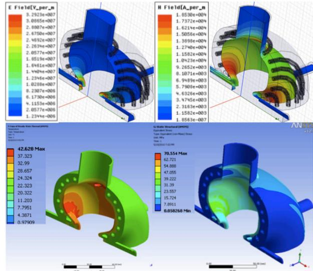
Figure 4: (Top) HFSS model showing cathode electric field of 20 MV/m (left), and surface magnetic field (right). (Bottom) Ansys model of the cavity temperature (left) and stress (right) distribution at  $P_{ave}=36$  kW
