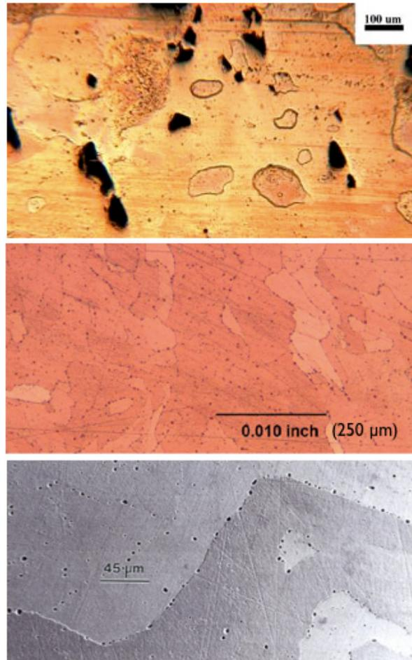
Figure 2: Micrograph of the initial high purity copper sample (top) and lower purity copper sample (middle and bottom) at different magnifications.
