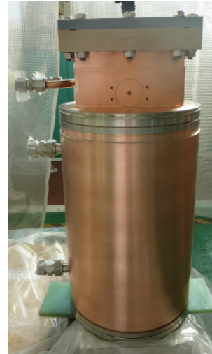
Figure 7: Duct-shaped SiC dummy load
