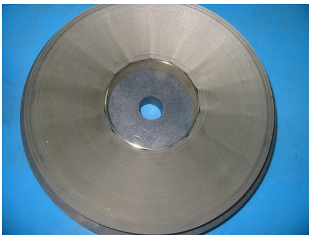
Figure 2: FT3L MA core with 27 cm diameter.[8]
