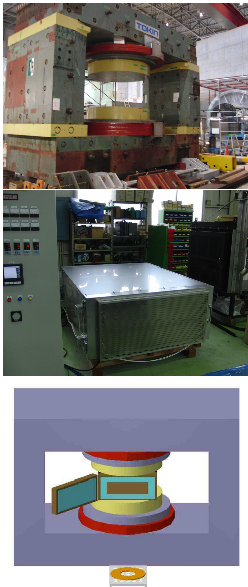
Figure 4: Top: FM Cyclotron Magnet, Middle:Oven to anneal FT3L material for J-PARC accelerators, Bottom:The oven will be installed in the FM Cyclotron magnet in this fall.
