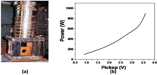
Figure 4: (a) Re-buncher I cavity (b) RF power vs. pickup voltage measurement plot for Re-buncher-I.
