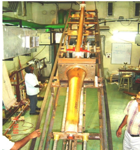
Figure 4: DEE stem brazing fixture.
