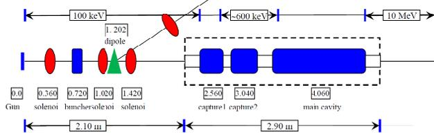
Figure 1: Injector schematic.
