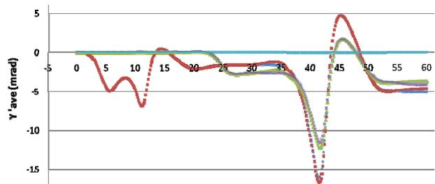
Figure 2: steering versus distance (cm) in capture section. u-d (blue), u-u (red), d-u (green), d-d (brown), none (cyan).
