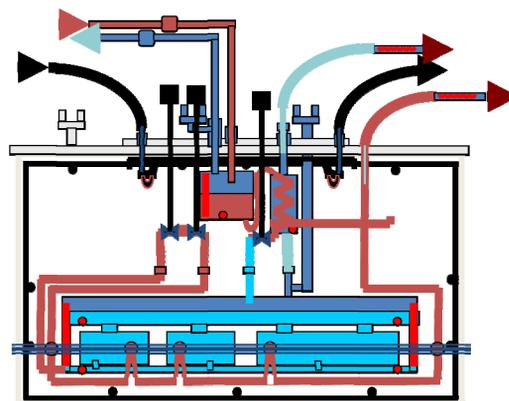
Figure 4: Top-load, box-type ICM with phase separator, 2K heat exchanger and JT expansion valve.
