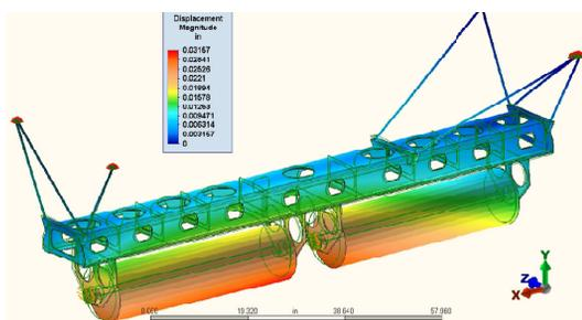
Figure 3: Cold mass (cavity string and 2 phase He pipe) supported from strong back slung from the ICM lid.
