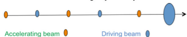
Figure 4: Scheme for beam loading and energy replacement in a DWA with interspersed pulse trains.
