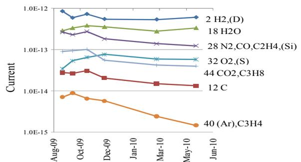
Figure 6: Long term residual gas components during conditioning. Note that the duty factors and voltage levels are not the same as the condition has been getting better.
