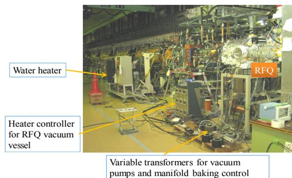
Figure 3: Baking of the RFQ.
