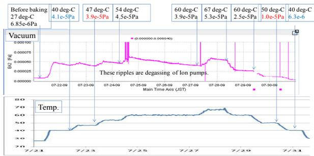
Figure 4: Vacuum pressure and temperature during the baking process.
