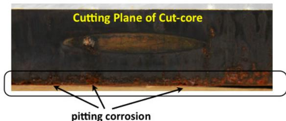
Figure 5: Pitting corrosion on the surface of the cut-core.
