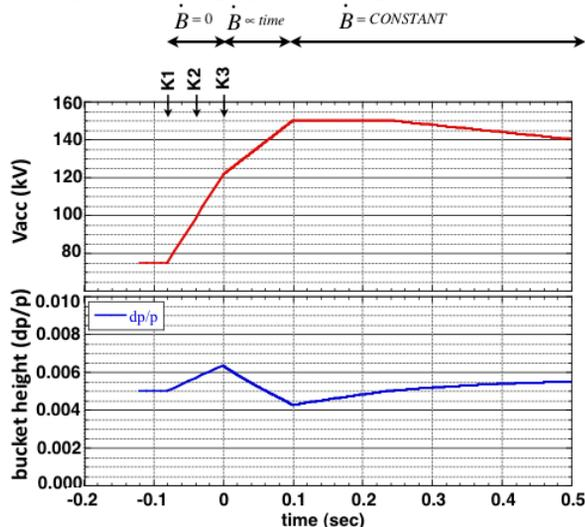
Figure 3: Typical RF voltage pattern and the bucket height (dp/p) near beginning of acceleration. Beam injections are at K1, K2, K3, and acceleration starts at  $t=0$ . Bending field is parabolically ramped between  $t = 0 \sim 0.1$  sec and  $B\dot{}$  is constant  $t > 0.1$  in Figure.
