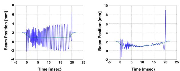
Figure 1: Beam phase plot during the whole acceleration. (Left): Phase Feedback OFF (Right): Phase feedback ON
