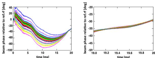
Figure 2: Beam phase plot during 1-hour 300kW operation (190 shots plotted). (Right): magnified (19 – 20ms).
