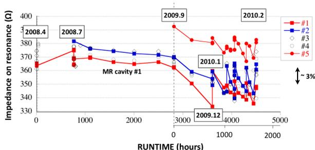
Figure 4: Trend graph of MR cavity impedance. All impedance measurements show the tendency to decrease since 2009.9
