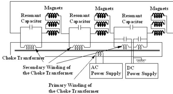
Figure 6: Resonant network of the KEK-DA magnets.
