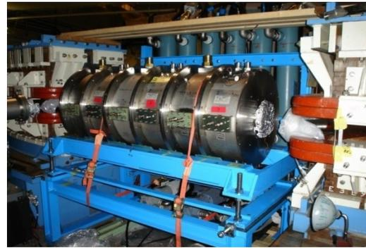
Figure 9: An assembly of 6 induction cells.
