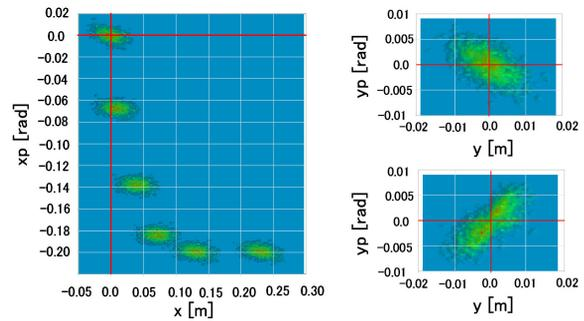
Figure 5: Phase space distributions of the beam. Left: in horizontal direction through the injection and Right: just at the deflector end.
