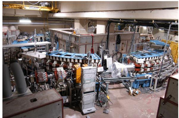
Figure 1: Photograph of the KEK-DA, It consists of 8 FDF combined-type magnets. Machine parameters:  $C_0=37.7$  m.  $B_{\max}=1.1$  T,  $f=10$  Hz,  $V_{\text{acc}}<3.2$  kV,  $v_x/v_y=21.1/2.3$ .
