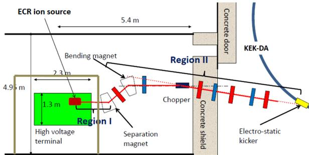
Figure 3: High voltage ion source and LEBT.
