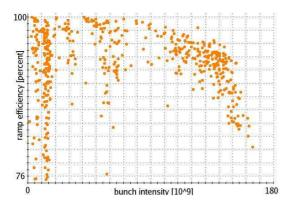
Figure 4: Ramp efficiency in the "Yellow" ring as function of injected bunch intensity.
