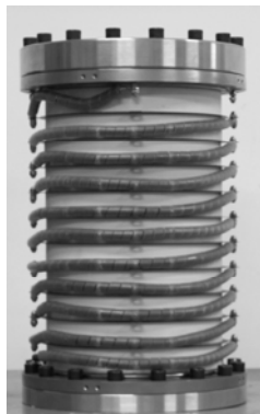
Figure 3 Structure of the accelerating tube
