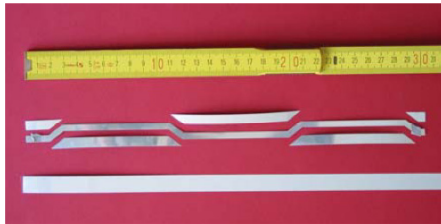
Figure 2: Single strand of Roebel cable. [8]
