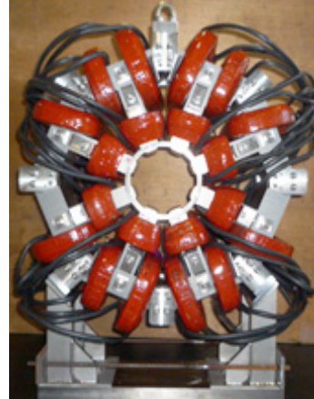
Fig. 6: The first magnet (not completed). The octupole and quadrupole coils were set in one coil package.
