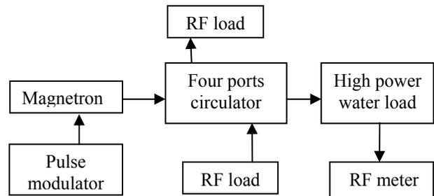
Figure 6: Experiment block diagram of high-power set.
