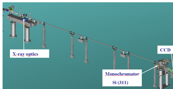
Figure 1: Sketch of the diagnostics beamline starting from the entrance absorber.
