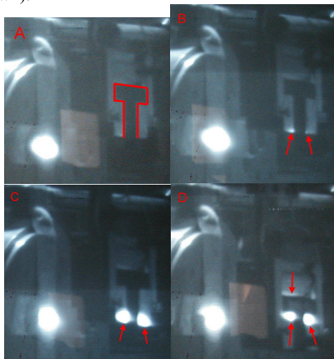
Figure 4. On slides B, C, D the VWM components exposed to the electron beam are highlighted. by the luminophor.
