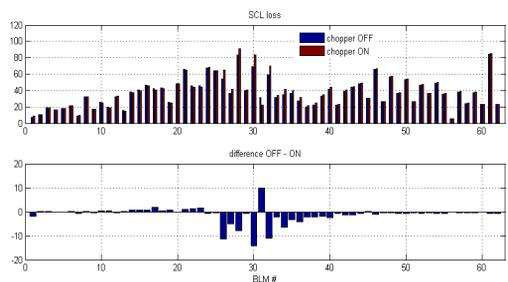
Figure 8: Effect of the MEBT chopper on beam loss in the SCL. An average loss increase of  $\sim 3\%$  is observed.
