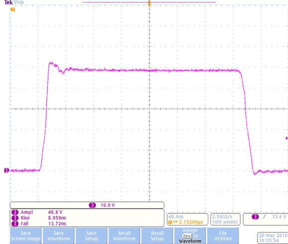
Figure 3: A high voltage pulse from the power supply measured on a 50 Ohm load.
