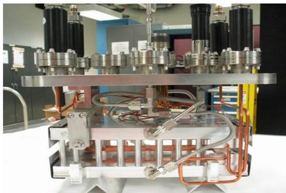
Figure 1: The new MEBT chopper deflector ready for installation.
