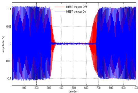
Figure 4: A gap in the beam created by the LEBT chopper (red) and cleared by the MEBT chopper (blue).
