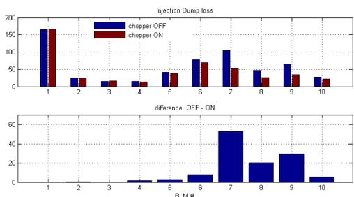
Figure 9: Effect of the MEBT chopper on beam loss in the ring injection. A loss reduction of  $\sim 20\%$  is observed.
