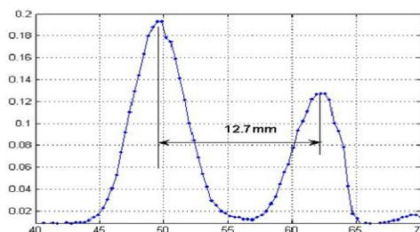
Figure 2: Transverse beam profile in front of the chopper target. The separation of chopped and un-chopped beamlets is proportional to the deflector kick strength.
