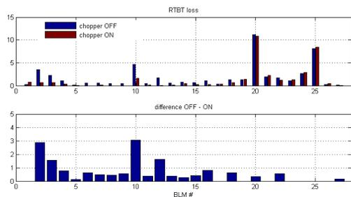
Figure 11: Effect of the MEBT chopper on beam loss in the RTBT. An average loss reduction of  $\sim 28\%$  is observed.
