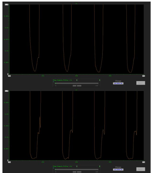
Figure 6: The beam gap depth measured using a logarithmic amplifier. The top snapshot is with the MEBT chopper off; the bottom snapshot is with the MEBT chopper on. Peak beam current is 40mA. The vertical scale is 5μA/div.
