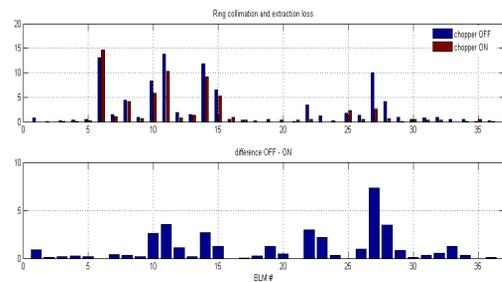
Figure 10: Effect of the MEBT chopper on beam loss in the extraction and collimation areas of the proton accumulator ring. An average loss reduction of  $\sim 35\%$  is observed.
