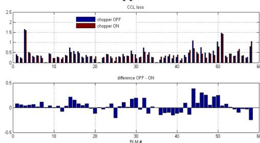
Figure 7: Effect of the MEBT chopper on beam loss in the CCL. An average loss reduction of  $\sim 2.5\%$  is observed.
