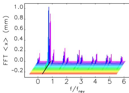
Figure 2: Evolution of Fourier transform of bunch-by-bunch horizontal centroids over 5000 turns, showing growth at  $1 - \nu_x$  in the absence of transverse feedback.
