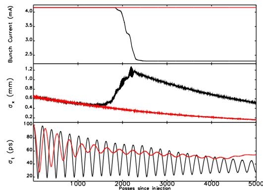
Figure 5: Turn-by-turn bunch current, bunch length, and bunch horizontal size for first (black) and 24<sup>th</sup> bunches filled in a 48-bunch uniform fill, using 10,000 particles per bunch.
