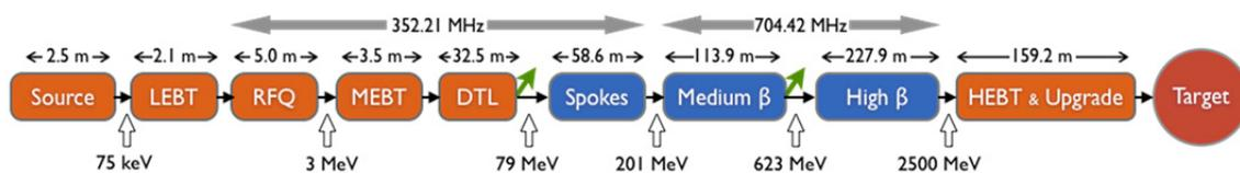
Figure 1: Schematic layout of the ESS linac [4]. Blue colour represents superconducting sections and green arrows locations where the beam could be extracted at intermediate energies.
