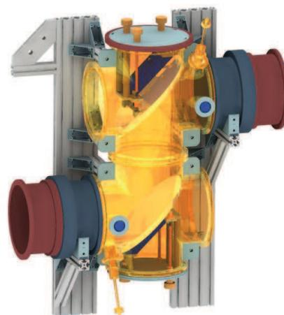
Figure 5: Design of a refocusing module consisting of a focusing and a flat mirror assembly. The vacuum chambers are made (yellow) transparent to show the mirrors and adjustment mechanisms.
