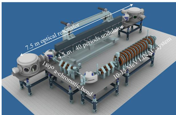
Figure 1: 3D design of the Nijmegen THz-FEL, showing LINAC, electron beam transport system, and optical cavity including 4.5 m long undulator.
