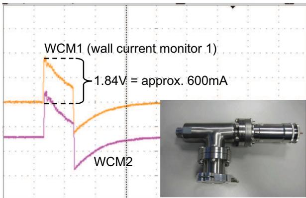
Figure 2: Proof-of-principle experiment: Oscilloscope trace of wall-current monitor signals showing that the 3 GHz modulated source can provide currents of 600 mA. The inset at the lower-right shows a photo of the source with connected matching circuit (right-hand side of the photo).
