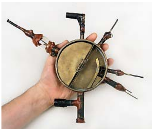
Figure 2: The 4-inch cyclotron vacuum chamber, showing the single dee, the deflector, and G. Seaborg's left hand.
