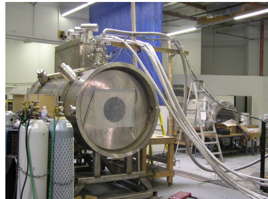
Figure 13: One of the spectrometer solenoid magnets is being tested at the fabrication company.
