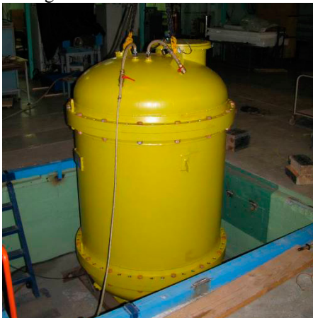
Figure 3: Pressure vessel used for HV section testing.
