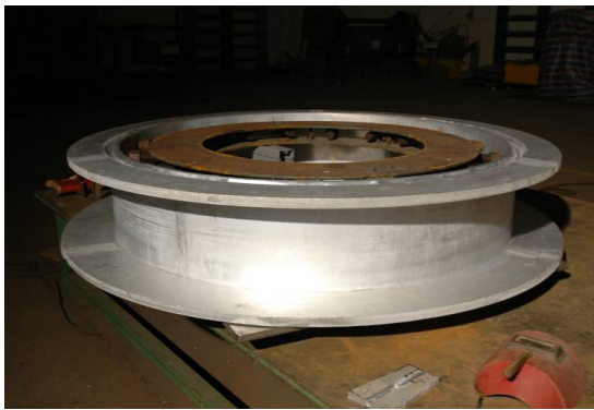
Figure 11: Coil mandrel under welding.
